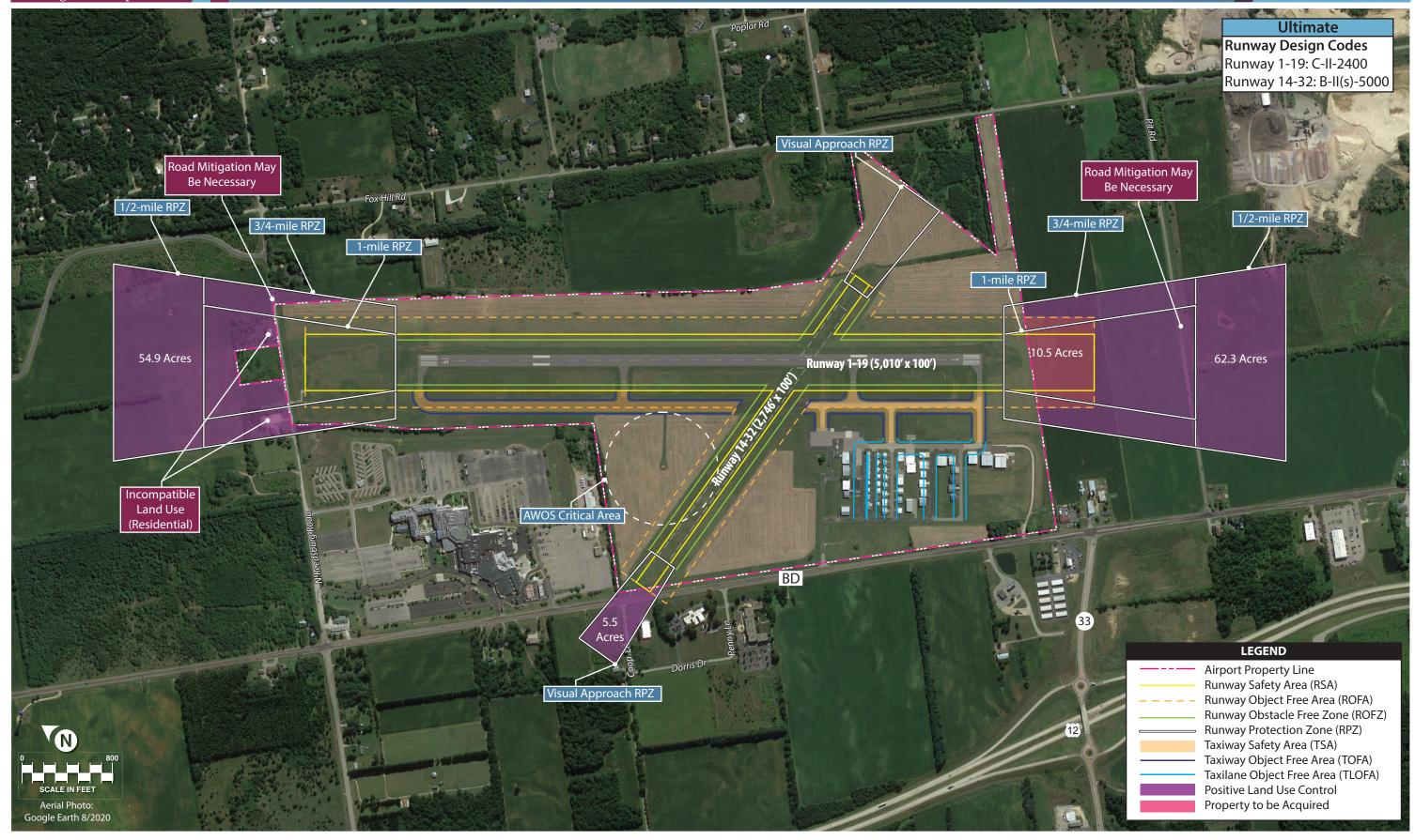
The exhibit shows that, by upgrading the RDC of Runway 1-19 from B-II to C-II and lowering the instrument visibility minimums to ½-mile, the amount of uncontrolled land uses within the runway RPZs increase to approximately 123 acres, without considering any extension to the runway. **Table 4C** lists the dimensions related to each approach RPZ based on the RDC and visibility minimum for each runway.
